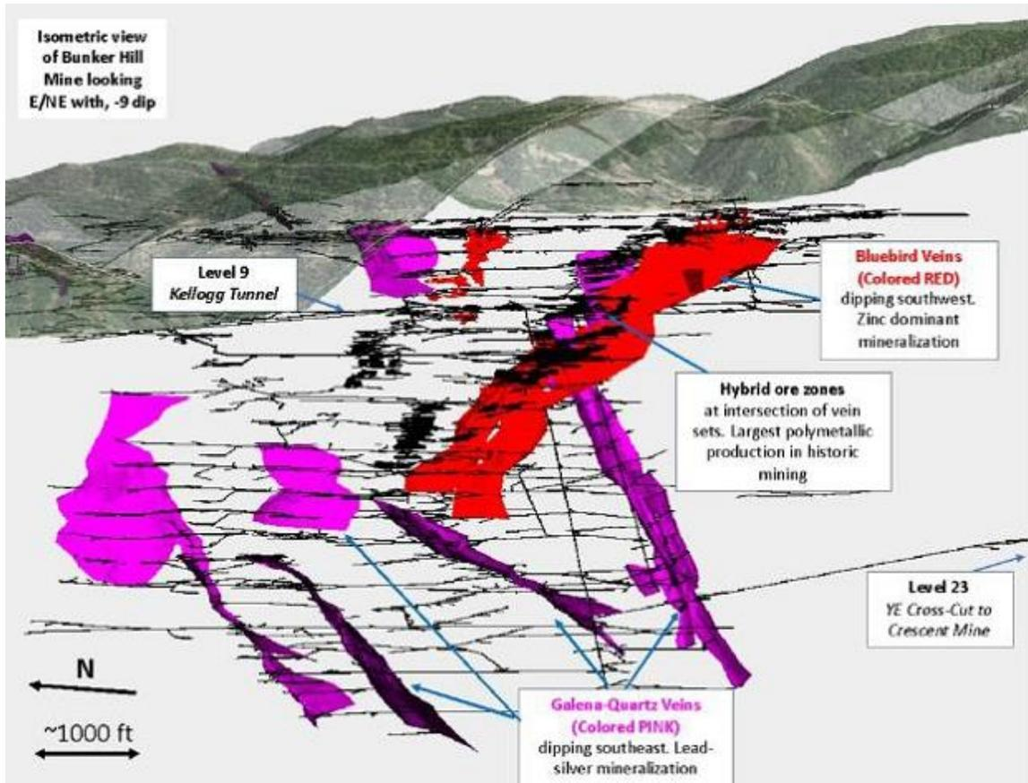
**Figure 6-11 Bunker Hill Mine workings with 3D vein models showing difference between Bluebird and Galena-Quartz Vein systems and location of hybrid mineralized zones.**
