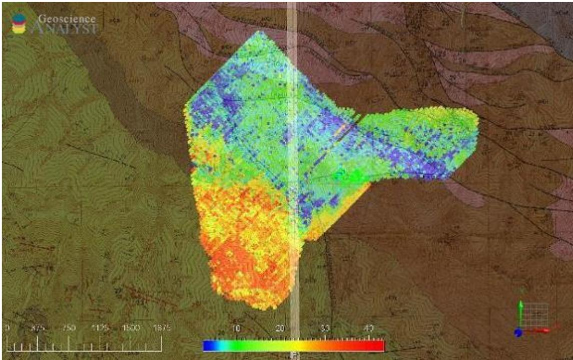
**Figure 7-6 Raw Dipole IP Data Over Compilation of Smeltonville and Kellogg 1965 USGS Geologic Quadrangle Maps Showing Correlation of IP Response and Lithology. Note IP Response to Major Mapped Fault Structures. Distance Scale in Meters, IP Scale in mVs/V.**
