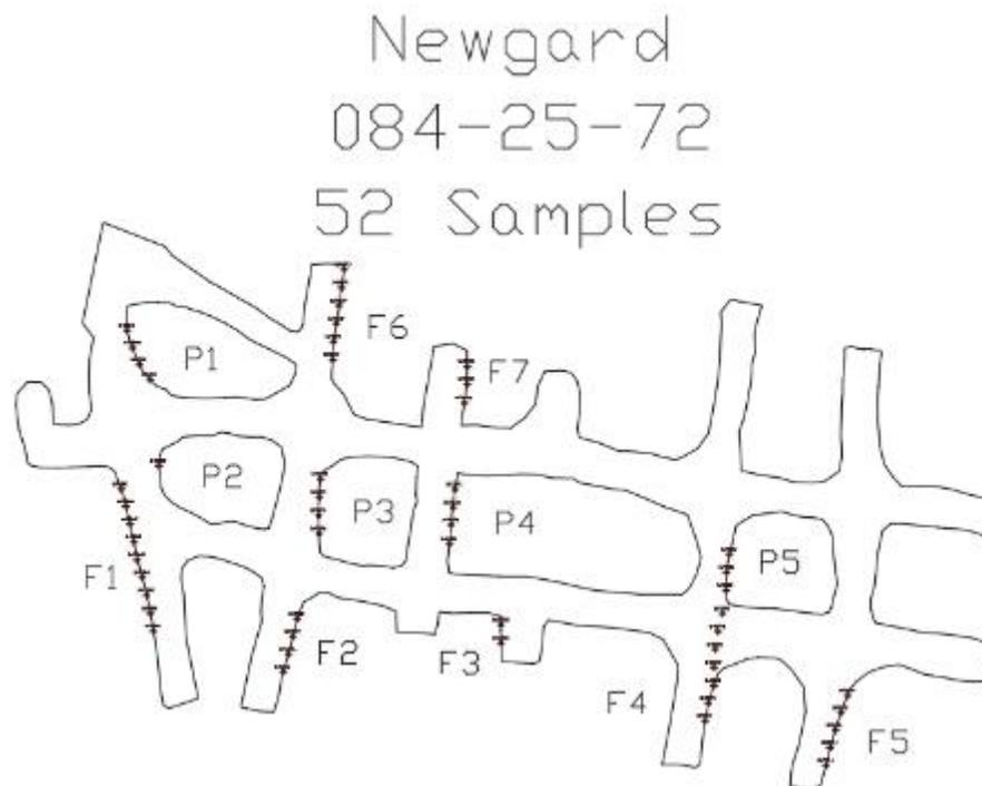
**Figure 9-5 Sample locations on the 084-25-72 sublevel using geo-referenced AutoCAD files**
