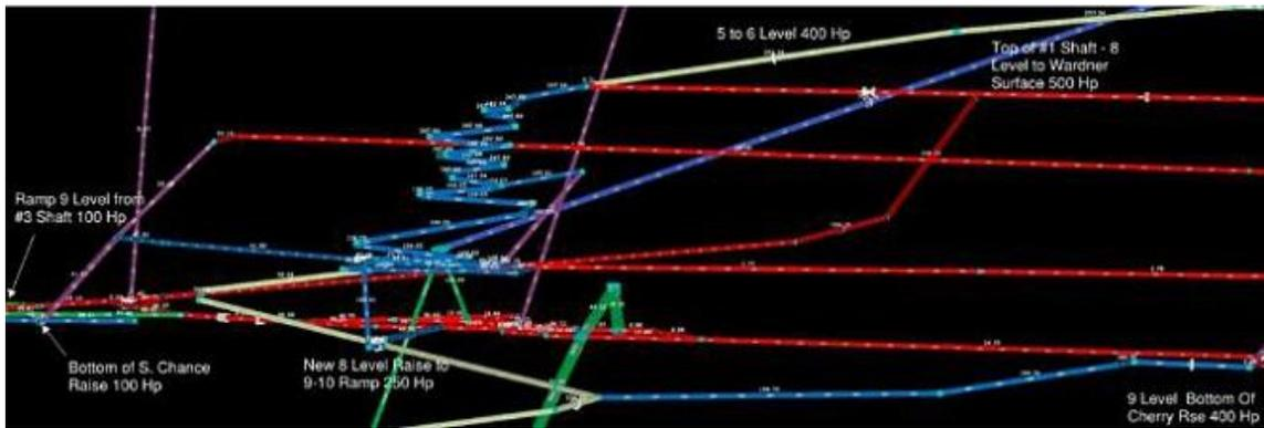
**Table 13-13 Isometric View of VNET Ventilation Model 5-level to 10-level (Looking Northwest)**
