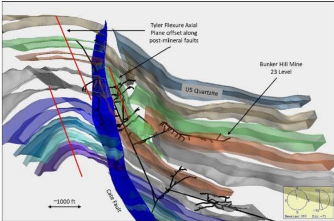
**Figure 6-8 Isometric view of Vulcan 3D model of L-0 through U-5 Quartzite units, looking nearly down-plunge on the Tyler Ridge Flexure axial plane, shown as red lines offset by faults. Only Cate fault is shown for simplicity.**
