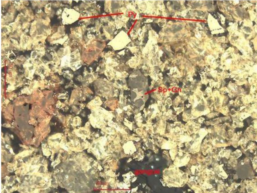
**Figure 10-6 BH LCT Zn Cleaner Concentrate Cyc 6 Area Photo Showing Yellow Sphalerite, Galena (Gn), Pyrite (Py) and Quartz Gangue - 200X RL**
