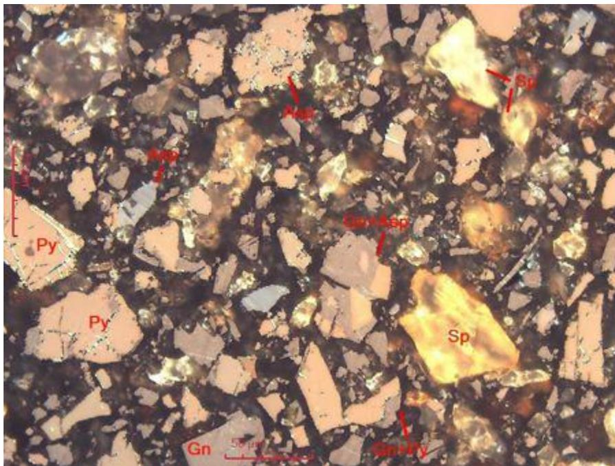
**Figure 10-5 BHFT 12 Pb Cleaner 3 Concentrate Area Photo Showing Galena (Gn), Pyrite (Py), Sphalerite (Sp) and arsenopyrite (Asp) - 200X RL**
