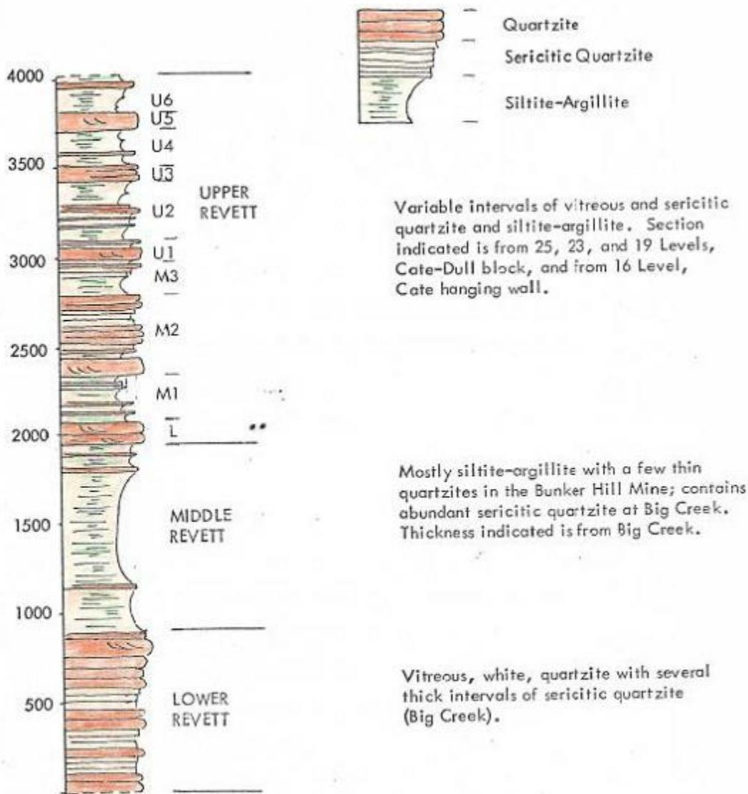
**Figure 6-6 Stratigraphic section of Revett formation in Bunker Hill area (White, 1976)**
