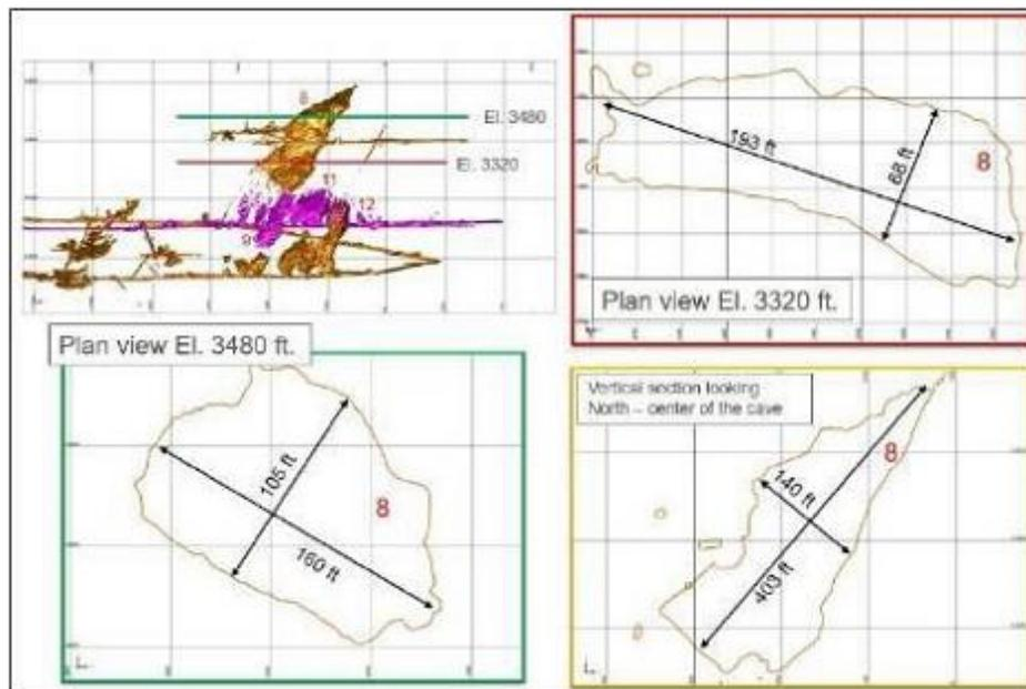
**Figure 13-5 Detail on 5-level McGatlin Stope (With Sections) Used for Span Analysis**
