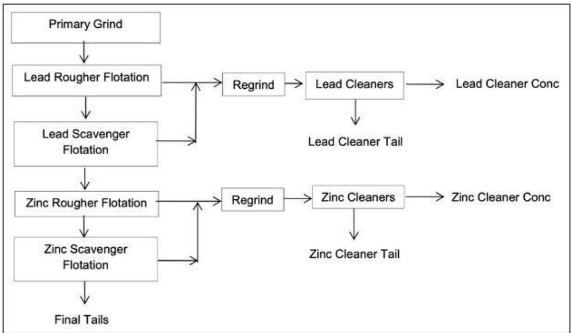
Figure 10-3 Cleaner Flotation Process Flowsheet (Tests 12-13)
