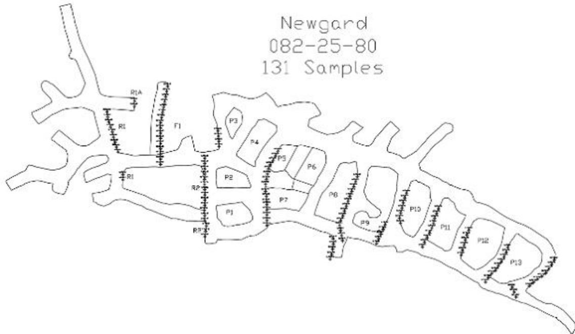
**Figure 9-4 Sample locations on the 082-25-80 sublevel using geo-referenced AutoCAD files**
