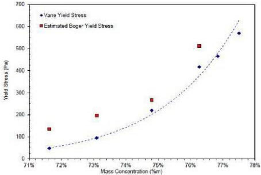
**Figure 13-8 Static Vane Yield Stress vs. Solids Mass Concentration**
