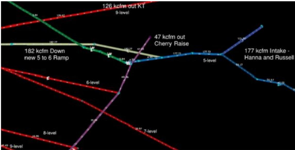
Figure 13-11 Isometric View of Upper-Level Vent Plan (Looking Northwest)
