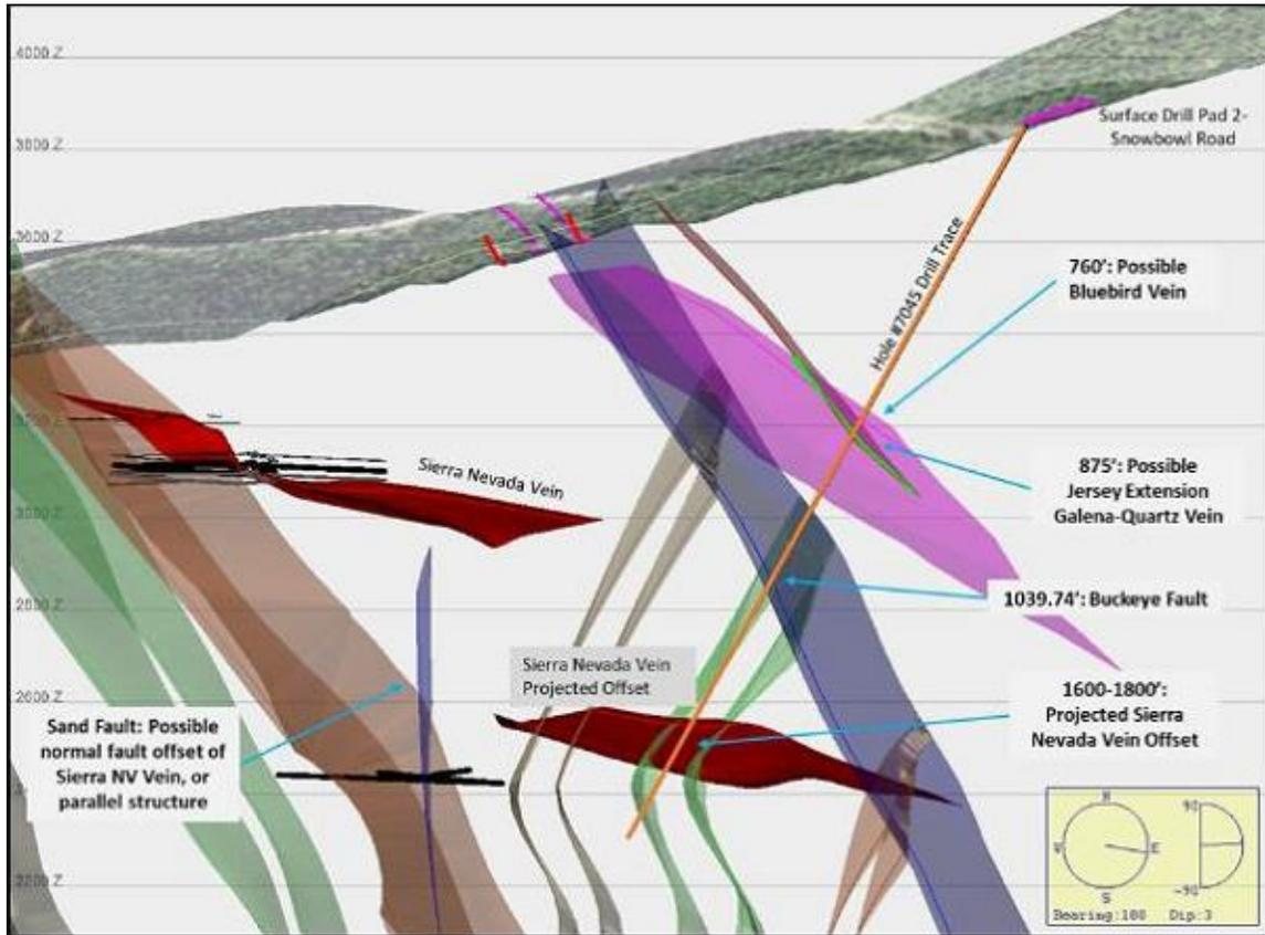
**Figure 7-3 Cross-section through Vulcan 3D models along planned drill hole trace showing expected downhole depths of projected geologic features. Historic Sierra Nevada Mine levels in black center right.**
