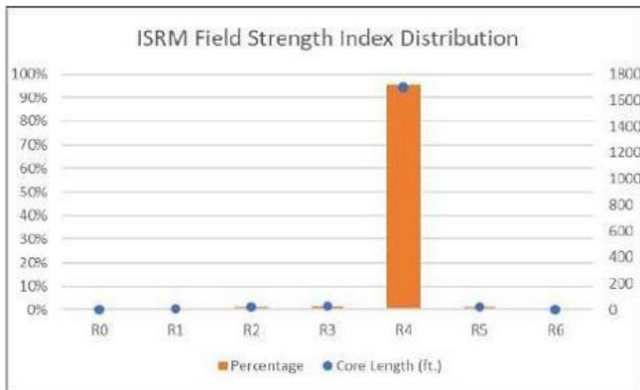
**Figure 13-6 ISRM Field Strength Index Distribution (in % and Core Feet Logged)**
