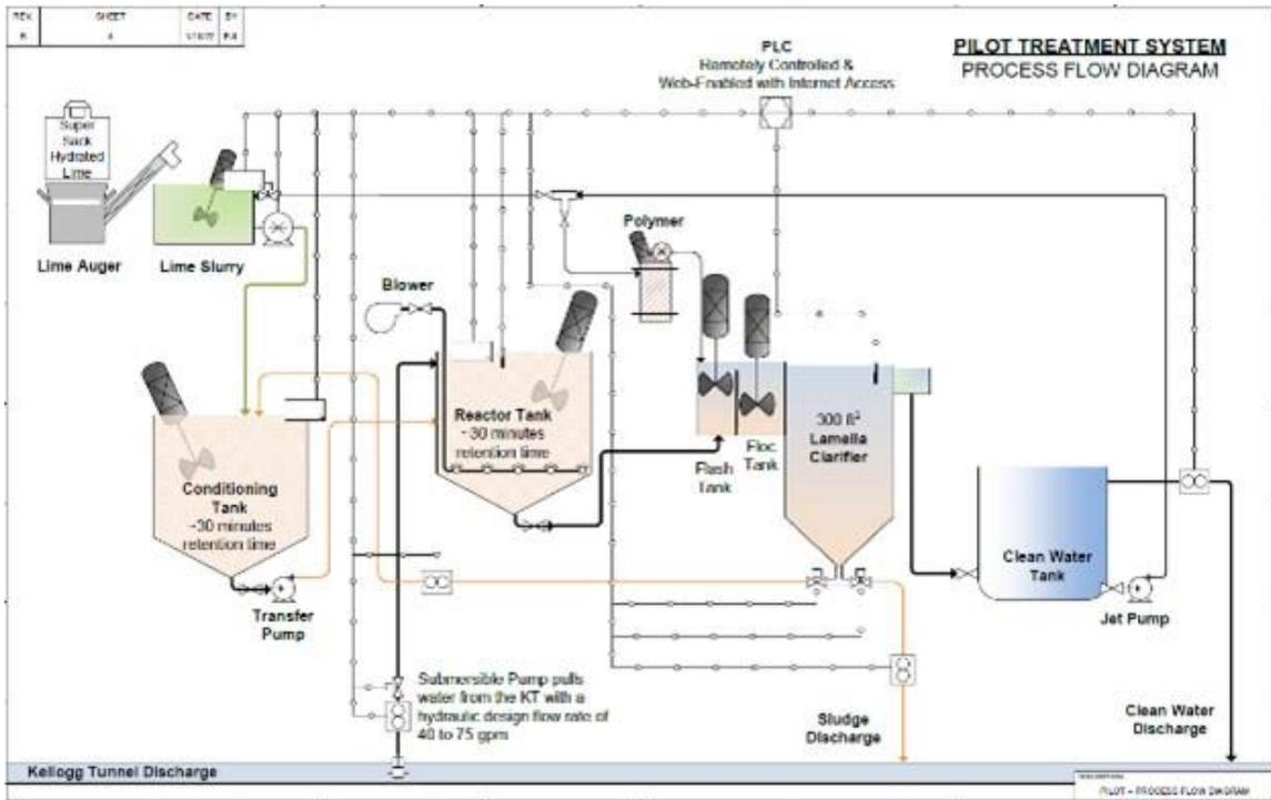
**Figure 17-1 Pilot Water Treatment Plant Process Flow Diagram**
