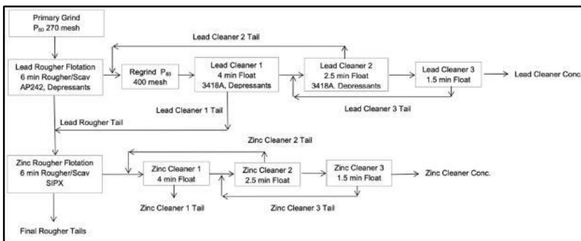
Figure 10-4 Locked-Cycle Test Process Flowsheet
