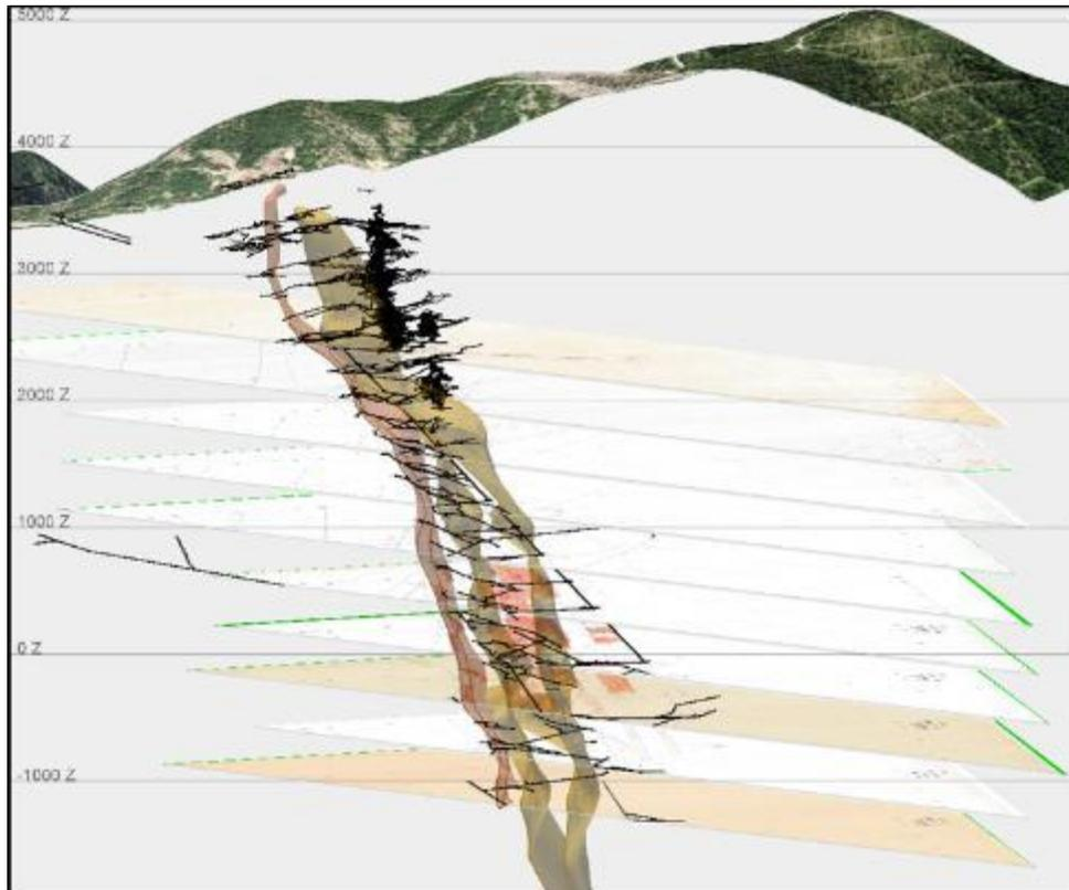
**Figure 7-1 1500 ft thick cross-section along BH #2 Shaft, looking at 106 azm, -12 degrees. Mine levels and shafts are black lines, thin dark orange shape between levels on left is 3D model of U-1 quartzite unit of the upper Revett formation, thick orange shape is M-3 siltite-argillite unit. Shapes built directly from original field mapping.**
