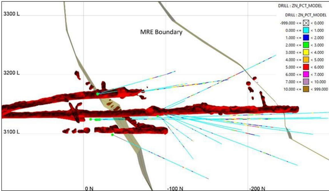
Figure 11-9 Section View DDH 7055 5-Level UTZ Looking SE (135°). 2020-2021 Drill Holes Zn%
