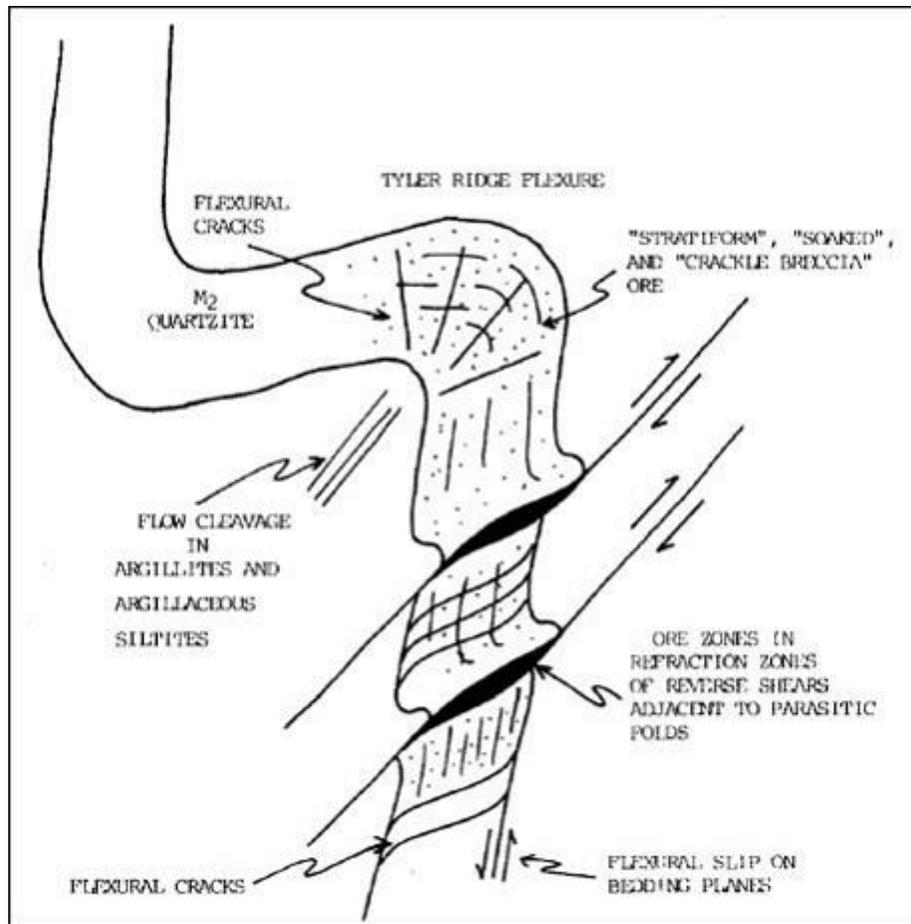
**Figure 6-9 Diagram of structural preparation of a quartzite bed from folding stresses (Juras and Duff, 2020)**
