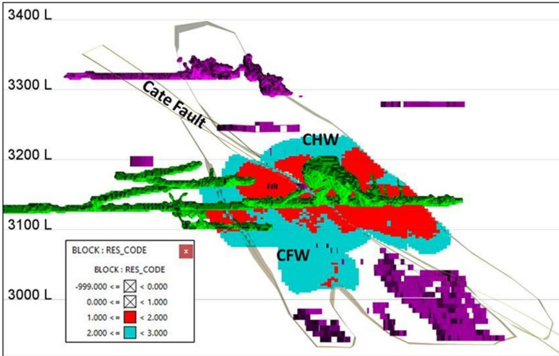
**Figure 11-15 Resource Classification for UTZ Model Sections. Section view looking N45E. Measured blocks shown in Red, Indicated blocks shown as Teal.**
