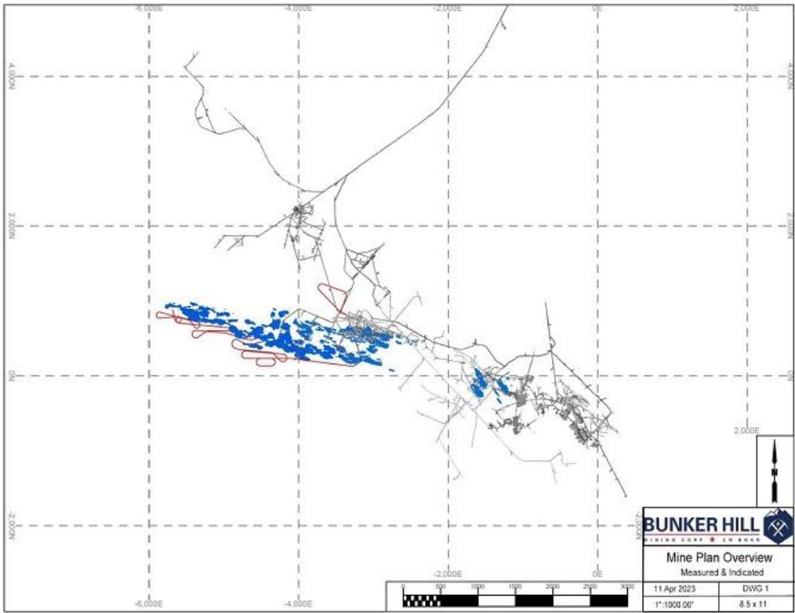
**Figure 13-9 Planned Mine Development and Production Stopes (with Currently Accessible Mine Drifts)**
