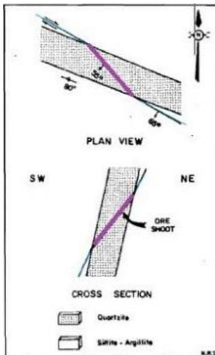
**Figure 6-12 Plan view and cross-sectional diagram of formation of mineralized shoot along vein in quartzite unit where rheologic contrast between argillite and quartzite causes refraction of vein surface (Juras, 1977)**
