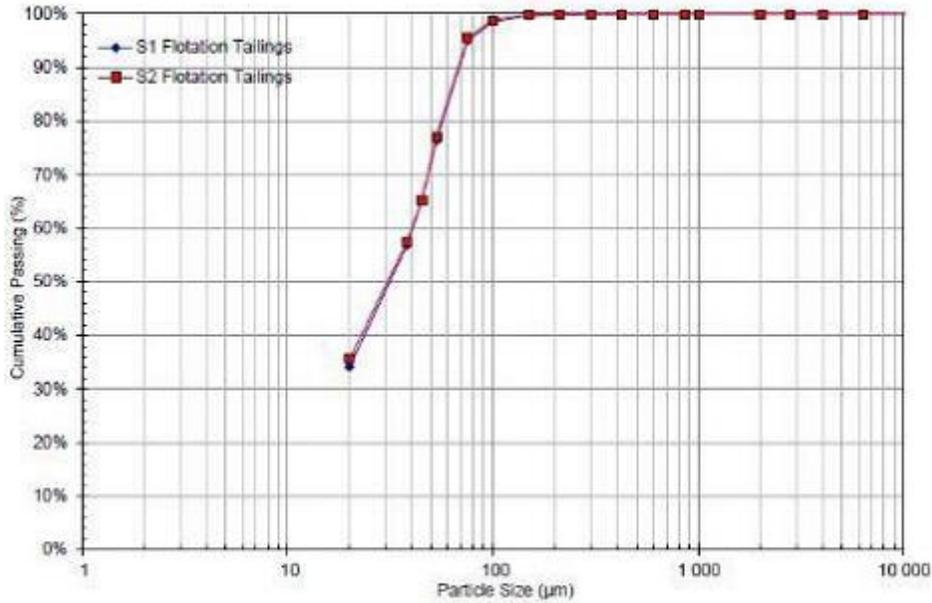
**Figure 13-7 Flotation Tailings Wet Sieve Particle Size Distribution**
