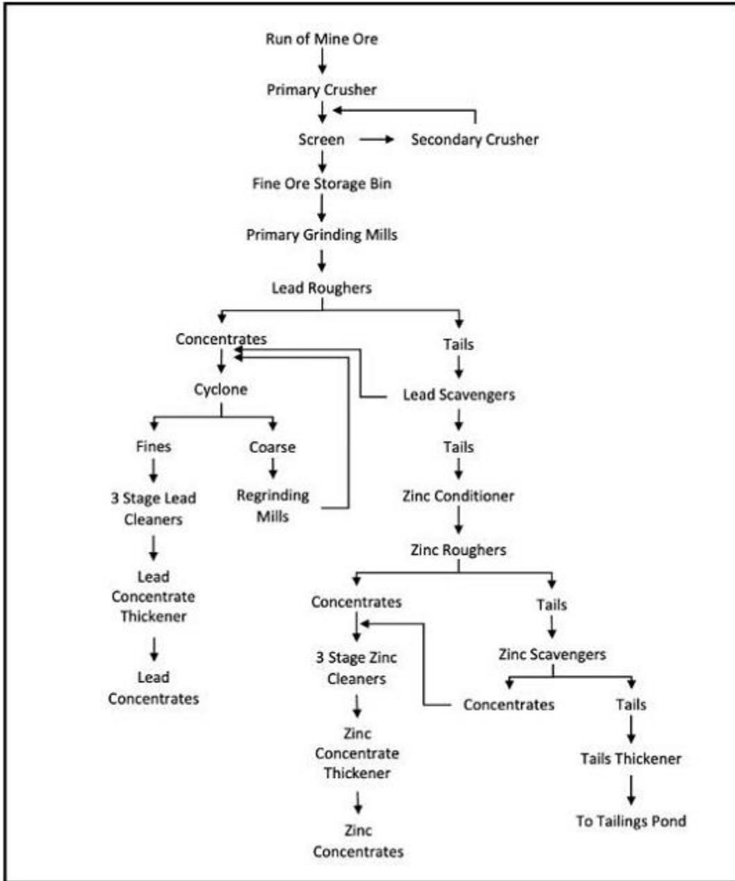
Figure 14-1 Bunker Hill Process Flowsheet
