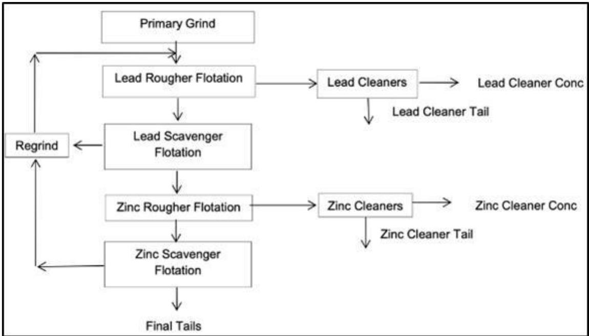
Figure 10-2 Cleaner Flotation Process Flowsheet (Tests 7-9)
