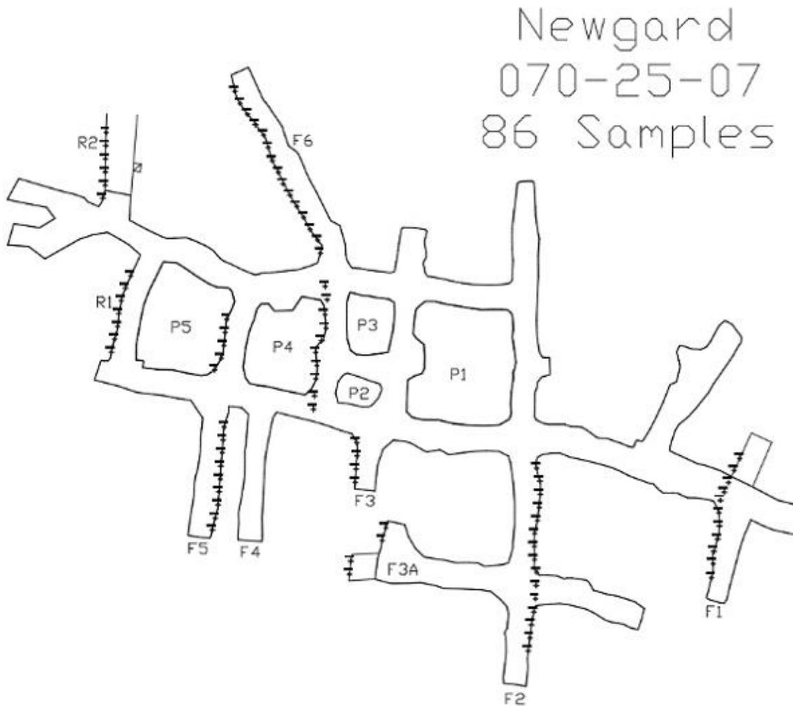
**Figure 9-3 Sample locations on the 070-25-07 sublevel using geo-referenced AutoCAD files**
