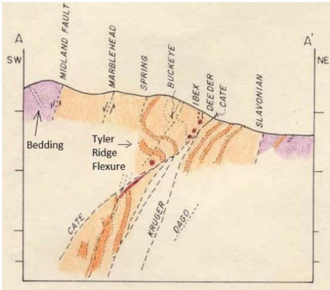
**Figure 6-10 Cross-section A-A' looking W-NW, not to scale (White and Juras 1976). Darker orange is quartzite bed in Upper Revett Formation.**
