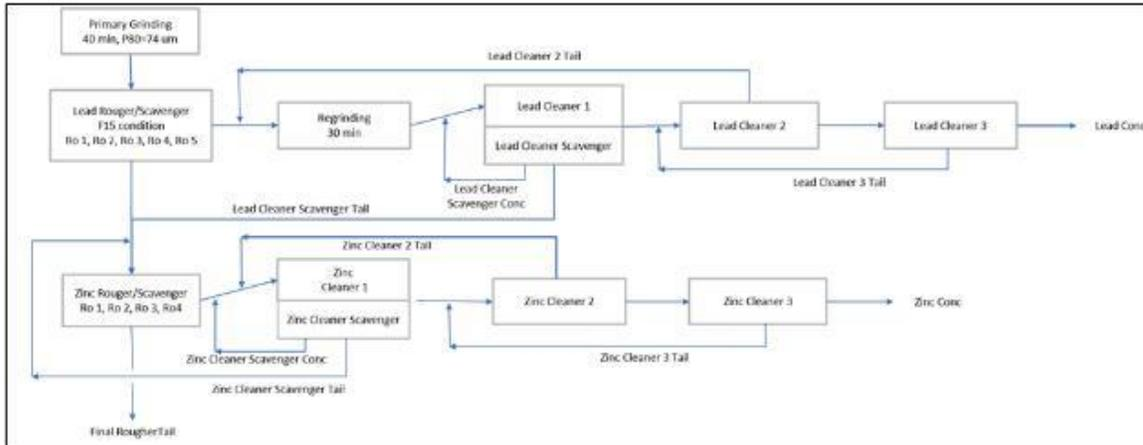
**Figure 10-7 Locked-Cycle Test Process Flowsheet (SGS 2022)**
