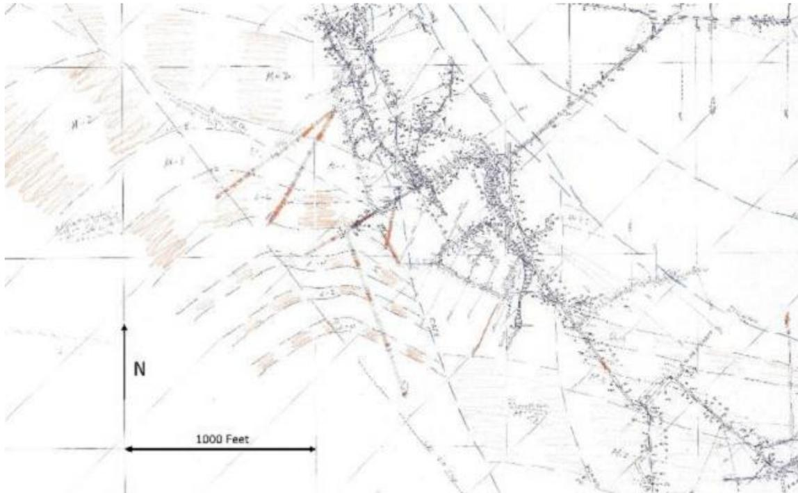
**Figure 6-7 Geologic Map of Bunker Hill Mine 17 Level showing quartzite units and exploration drill holes**
