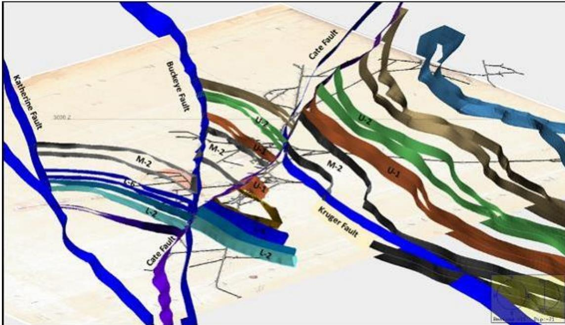
**Figure 7-2 Isometric view of plan section through 3D lithology and Fault Models at BH 9 Level. View is looking 311 azm, -21 dip, with 100' window on either side of stratigraphy map at 2405' elevation.**
