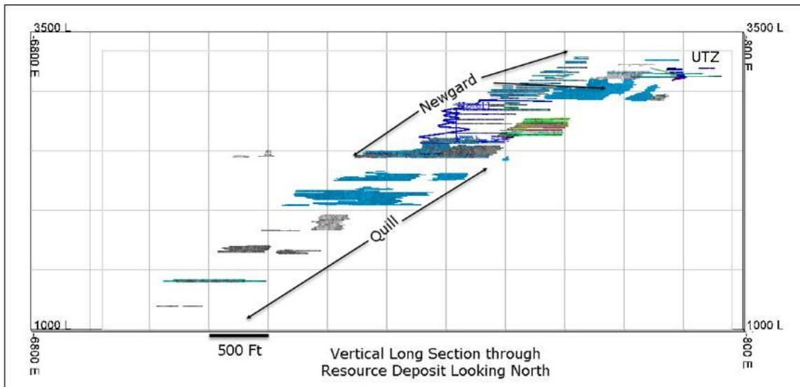
**Figure 11-2. Vertical long section through the deposit showing depleted stopes down-dip and mineralized pillars between stopes**
