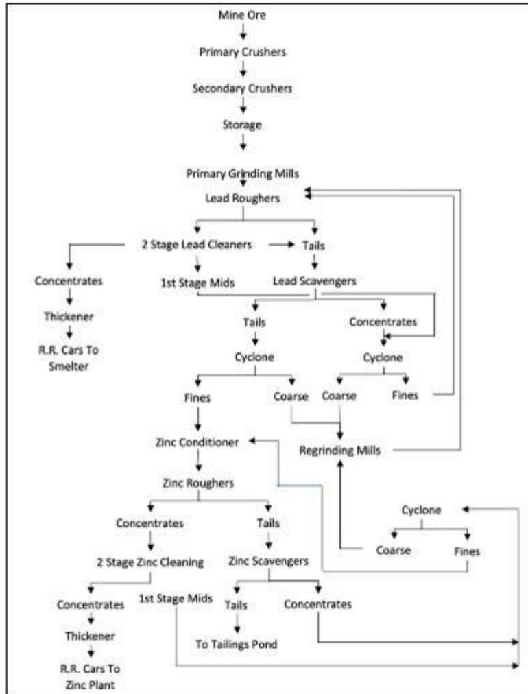
Figure 10-1 Historical Process Plant Block Diagram of the Bunker Hill Mining Concentrator
