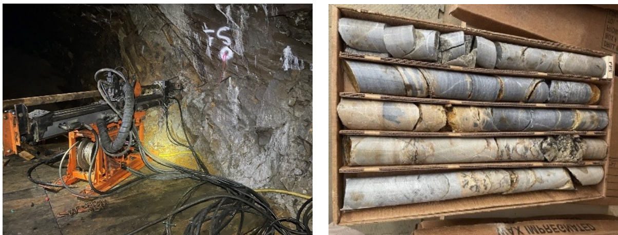
Figure 10: UG Drilling and core samples
