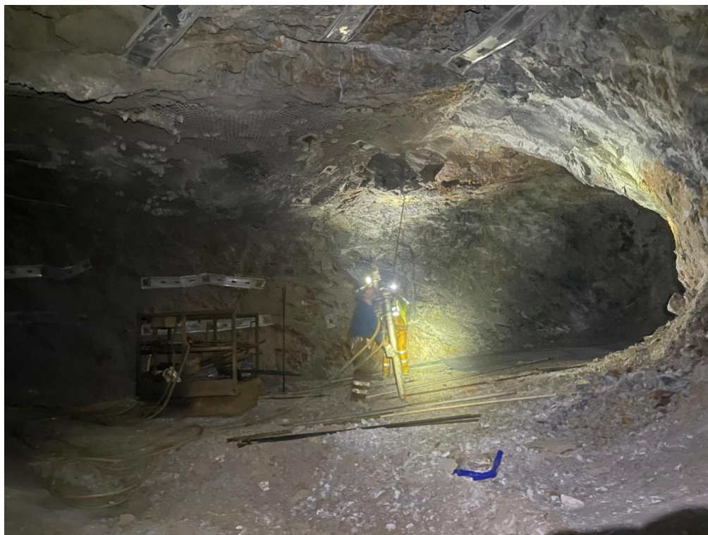
Figure 4 - Rehabilitation work on 8 Level, with ore collected during development work being stockpiled
