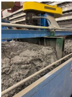
Lead Concentrate being floated in flotation circuit
