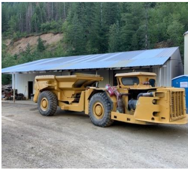
Photo 4: 16-ton haul truck
