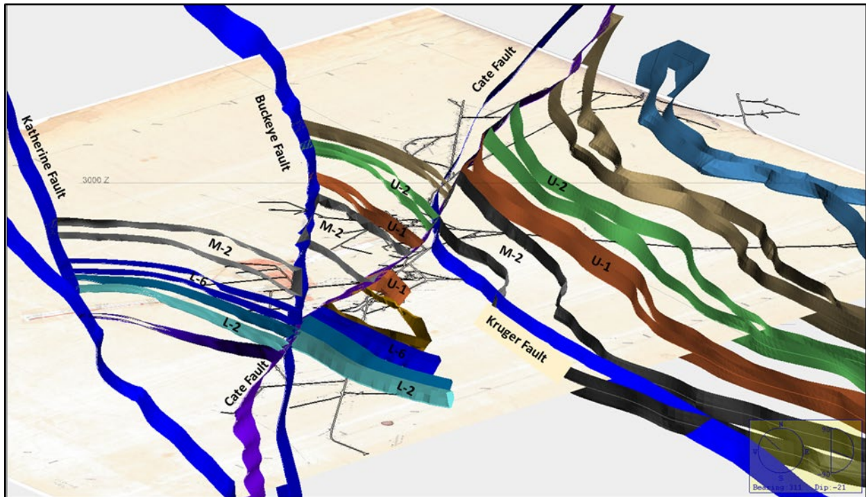
Figure 9-2 Isometric view of plan section through 3D lithology and Fault Models at BH 9 Level. View is looking 311 azm, -21 dip, with 100' window on either side of stratigraphy map at 2405' elevation.
